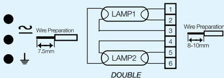
Strip the seven ends of output cable to be each 8 - 10mm
